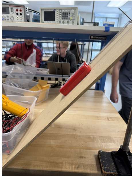
Figure 14: Picture for the set up of the 60° in lab. The wooden board was propped up against the retort stand at an angle of 60 degrees. The same bolt attached to the wooden board as in part 1 was used to attach the spring and iOLab. The iOLab oscillated diagonally on this wooden board with wheels down allowing it to roll freely.
