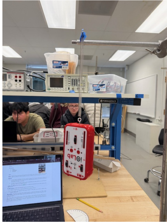
Figure 5: Picture of the set up for the 90^\circ in lab. The iOLab was suspended by a spring attached to the metal dowel and was dropped from rest allowing it to oscillate up and down freely.
